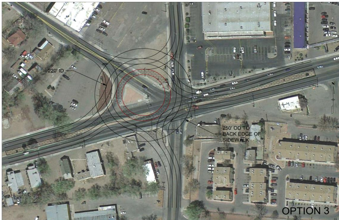
Bridge Boulevard and Sunset Drive/Five Points Road Recommended Roundabout Orientation
